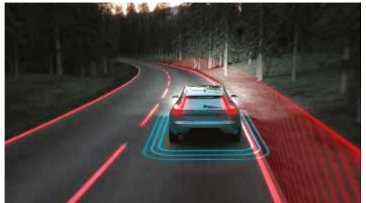
Run-Off Road Mitigation with Road Edge Detection
