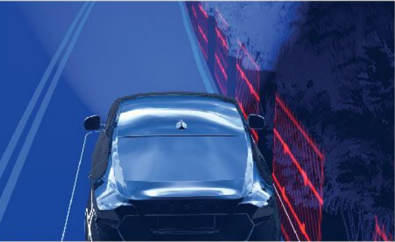
Run-off Road Mitigation with Road Edge Detection
